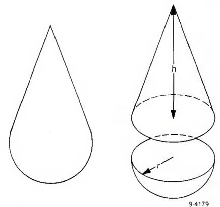
Fig. 8—Geometry used to calculate the effect of surface-tension-stored energy on the initial velocity of the drop.
