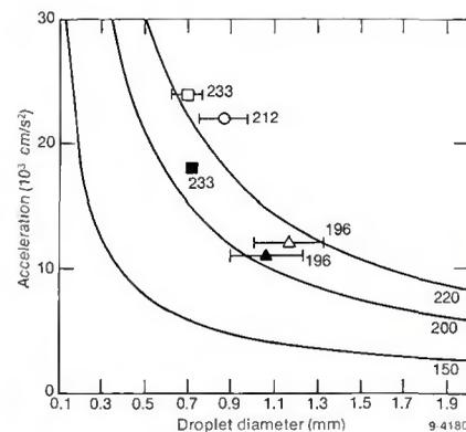
Fig. 7—Comparison of drop accelerations measured in this work with those derived from calculated plasma velocities by Lancaster. Currents in amperes.
