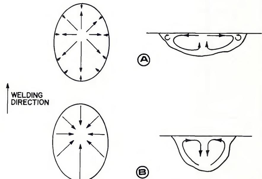
Fig. 1—Proposed fluid flow on and below the weld pool surface: A—negative surface tension temperature coefficient; B—positive surface tension temperature coefficient
