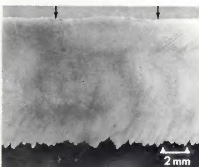
Fig. 11—Longitudinal section of a sharply focused electron beam weld crossing a selenium-doped, beam melted zone in 21-6-9. The Se-doped zone lies approximately between the arrows
