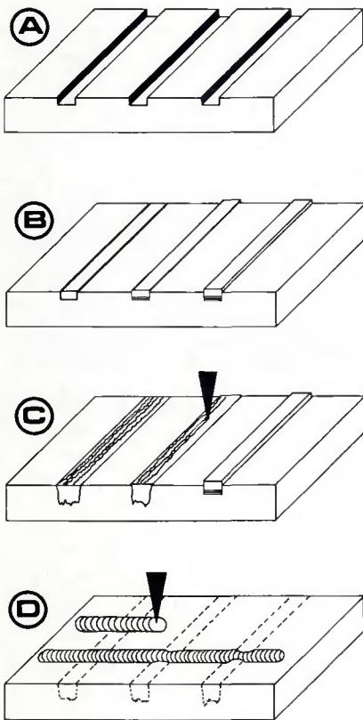
Fig. 2—Procedure for doping 21-6-9 base metal; flattening and milling the plate smooth are not shown. A—machine slots in surface; B—insert foil(s) and cover plates in slots; C—electron beam melt cover plates, foil(s), and some base metal; D—run GTA weld beads across electron beam melted zones
