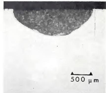
Fig. 3—Cross section of defocused, decoupled laser weld in undoped base metal with focus above 21-6-9 plate surface
