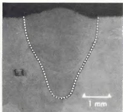
Fig. 10—Cross section of a defocused electron beam weld in a selenium-doped, beam melted zone in 21-6-9; fusion zone boundary outlined for clarity
