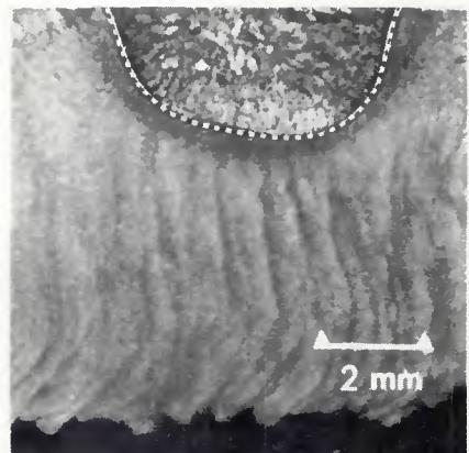
Fig. 6—GTA weld cross section in a sulfur-doped electron beam melted zone in 21-6-9 containing 80 ppm S; fusion zone boundary outlined for clarity
