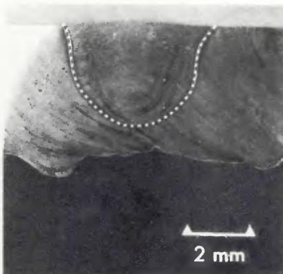
Fig. 8—GTA weld cross section in a tellurium-doped electron beam melted zone in 21-6-9 containing 62 ppm Te; fusion zone boundary outlined for clarity
