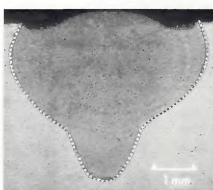
Fig. 12—Cross section of a defocused, coupled laser weld with the focus below the plate surface in 21-6-9; fusion zone boundary outlined for clarity
