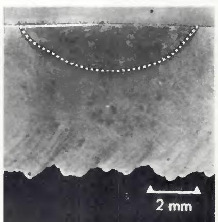
Fig. 7—GTA weld cross section in an undoped electron beam melted zone in 21-6-9; fusion zone boundary outlined for clarity
