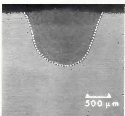
Fig. 13—Cross section of a defocused, decoupled laser weld with the focus below the plate surface in 21-6-9; fusion zone boundary outlined for clarity
