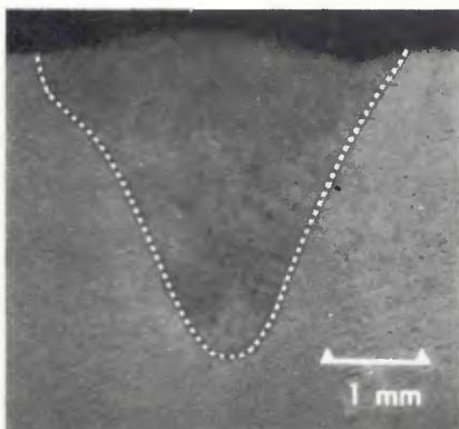
Fig. 9—Cross section of a defocused electron beam weld in an undoped, beam melted zone in 21-6-9; fusion zone boundary outlined for clarity
