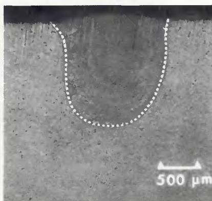
Fig. 4—Cross section of defocused, decoupled laser weld with focus above plate surface in a selenium-doped electron beam melted zone in 21-6-9; fusion zone boundary outlined for clarity
