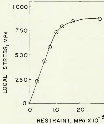
Fig. 2—Non-linearity in reaction stress vs restraint plot at high restraints for single pass weld (from Satoh, et al. 4 )
