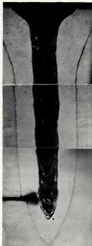
Fig. 4—Photomicrograph of weld shown in Fig. 3 made in U-0.75 wt% Ti. These two composite views are made from different exposures of the same negatives. Electrolytic etch with (8-5-5) plus air oxidation for 16 months
