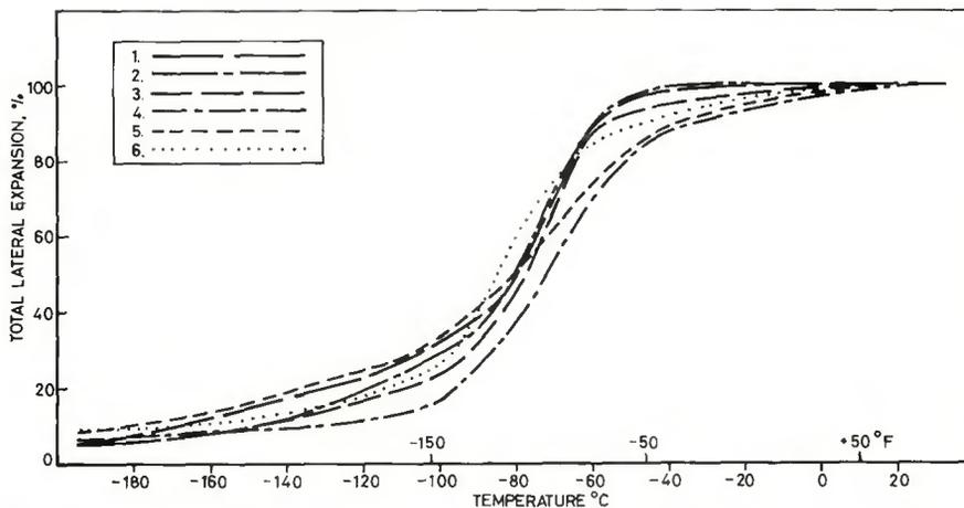
Fig. 8 — Variation in % lateral expansion with temperature
