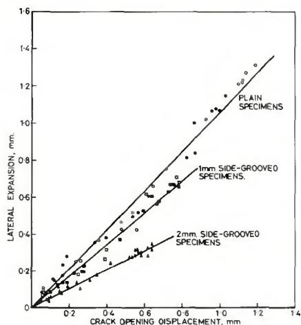
Fig. 5 — Relationship between crack opening displacement and lateral expansion
