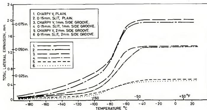
Fig. 1 — Variation in total lateral expansion for failure with temperature
