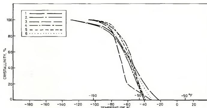
Fig. 4 — Variation in fracture appearance with temperature
