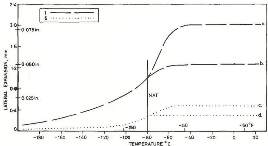
Fig. 11 — Variation in lateral expansion with temperature for specimen types 1 and 6; (a) lateral expansion for complete failure in specimen type 1; (b) lateral expansion for crack initiation in specimen type 1; (c) lateral expansion for complete failure in specimen type 6; (d) lateral expansion for crack initiation in specimen type 6
