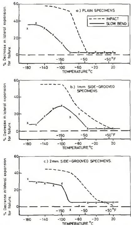
Fig. 6 — Influence of change in notch acuity from Charpy V to 0.15 mm slit on the lateral expansion for failure
