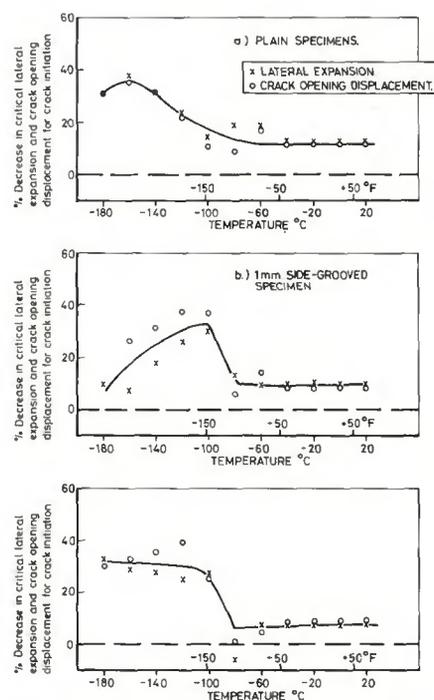
Fig. 7 — Influence of change in notch acuity from Charpy V to 0.15 mm slit on critical lateral expansion and crack opening displacement for crack initiation
