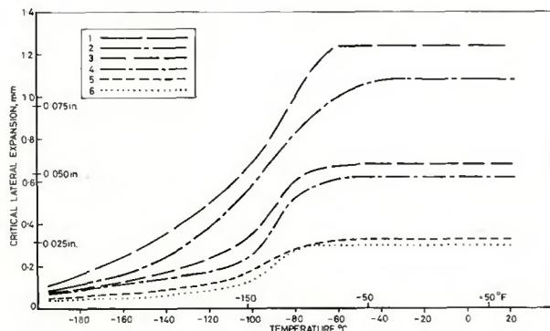
Fig. 2 — Variation in critical lateral expansion for crack initiation with temperature
