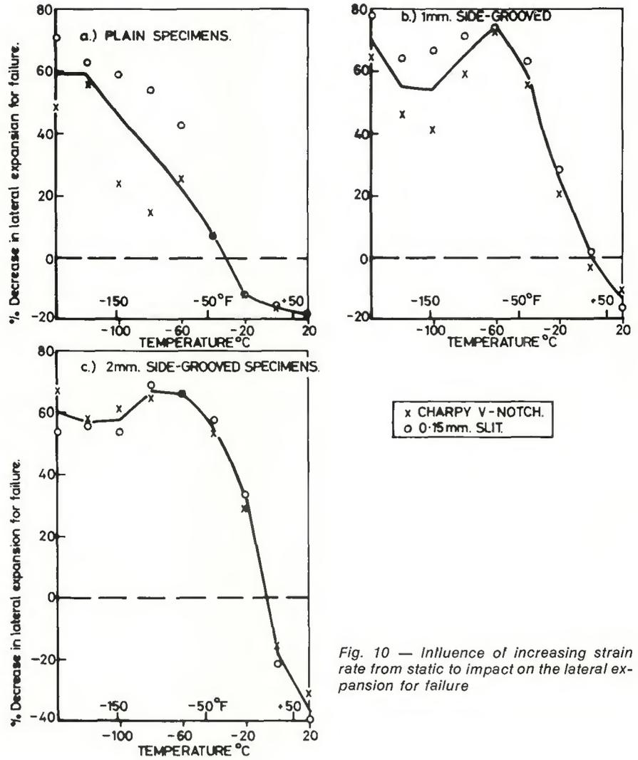
Fig. 10 — Influence of increasing strain rate from static to impact on the lateral expansion for failure
