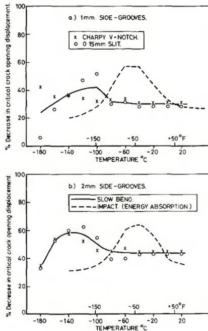
Fig. 9 — Influence of side grooving on critical crack opening displacement
