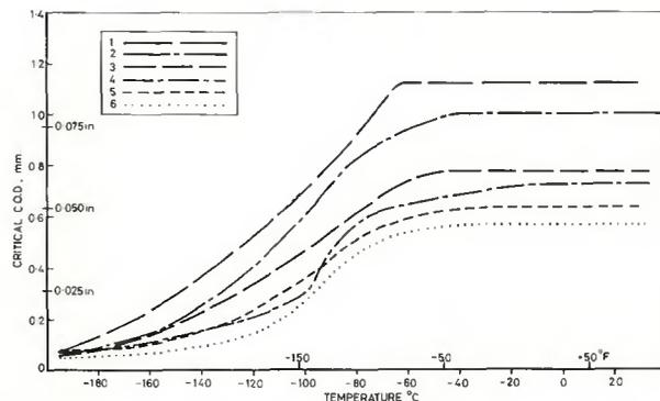
Fig. 3 — Variation in critical crack opening displacement for crack initiation with temperature
