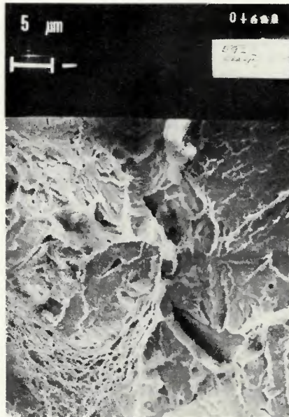
Fig. 11 — Scanning electron micrograph from Charpy V-notch specimen broken at -170 C, HY130 (reduced 51%)
