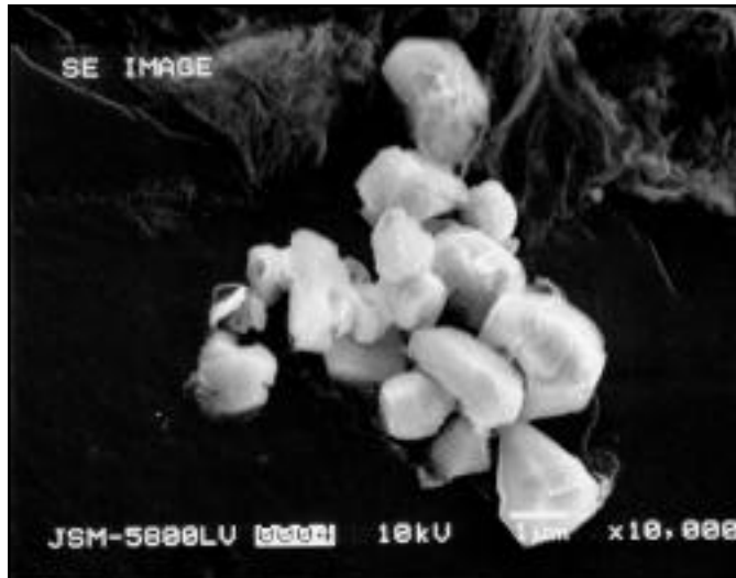
Fig. 6 — SEM micrograph of high-aluminum weld (E70T-4).
