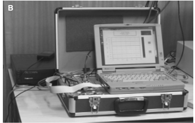
Fig. 8 — Experimental setup for specimen fabrication and data acquisition. A — Welding system for specimen fabrication; B — data logging system using WeldPrint software.
