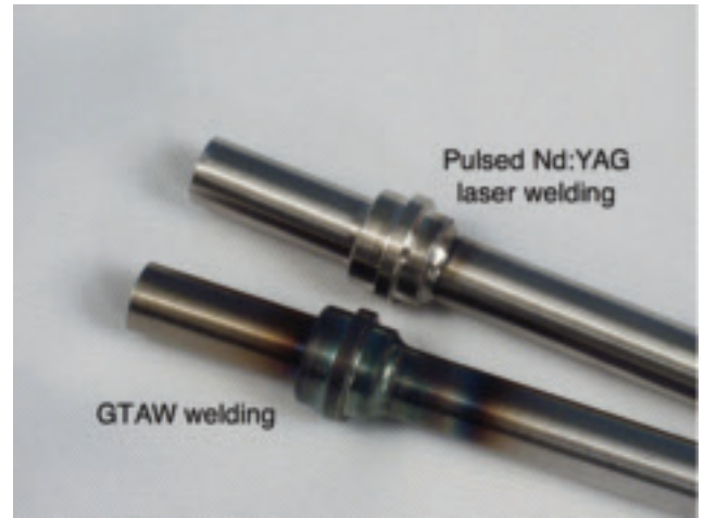
Fig. 2 — Laser beam welding and GTAW visual heat effects.
