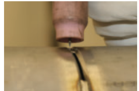
Example of proper arc length.
