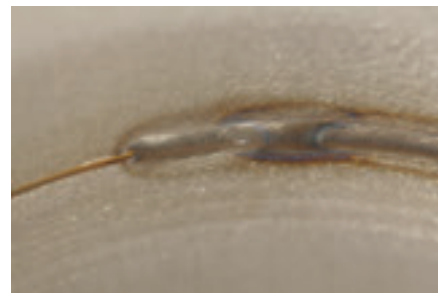
This “star” or crater crack occurred because the edge of the weld pool solidified before the center.
