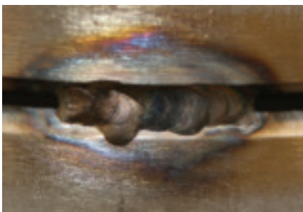
No backing gas: outside the pipe.
