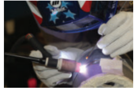
Set the gas postflow to 5 to 10 s longer than normal.
