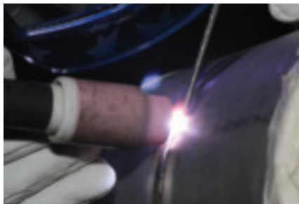
Keep the torch directed nearly straight at the joint.
