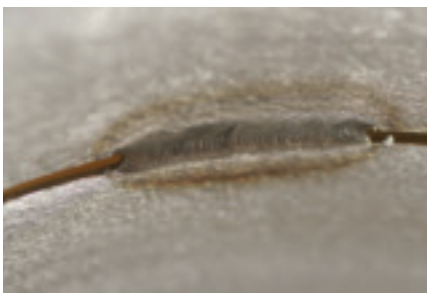
The inside of the same tack weld.
