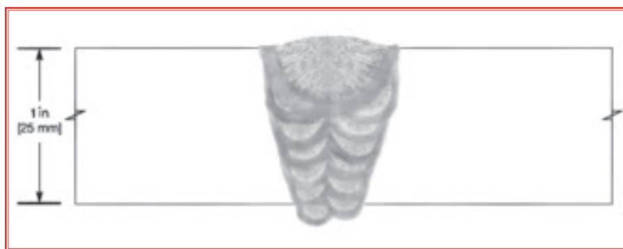
Fig. 1 — Cross section of multiple pass flux-electrode classification weld.
