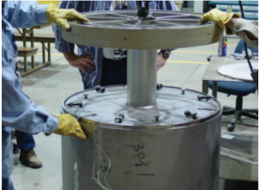
Fig. 3 — Shown are the thermocouple attachment locations and setup.
