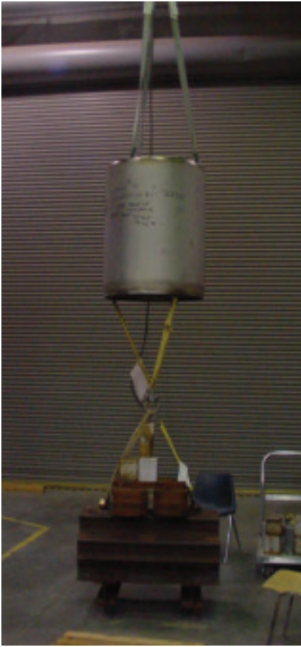
Fig. 2 — A pull test of 1.25 times the design lifting load took place on the overpack.
