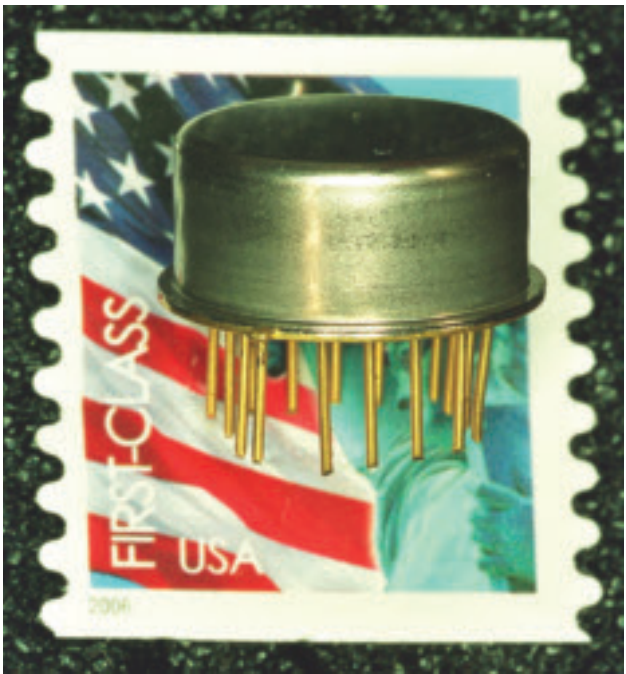
Fig. 2 — Vacuum-welded, 0.60-in.-diameter package.
