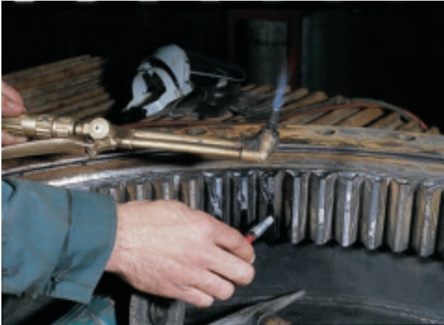
Fig. 2 — A temperature indicator is used to check the surface temperature on a gear.
