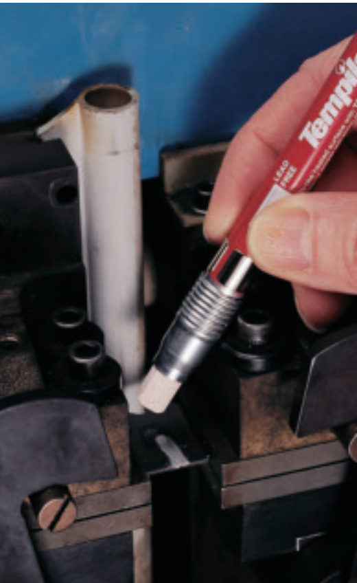
Checking the surface temperature of a custom alloy.
