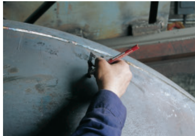
Fig. 4 — A welder uses a temperature crayon to mark a piece close to a weld.
