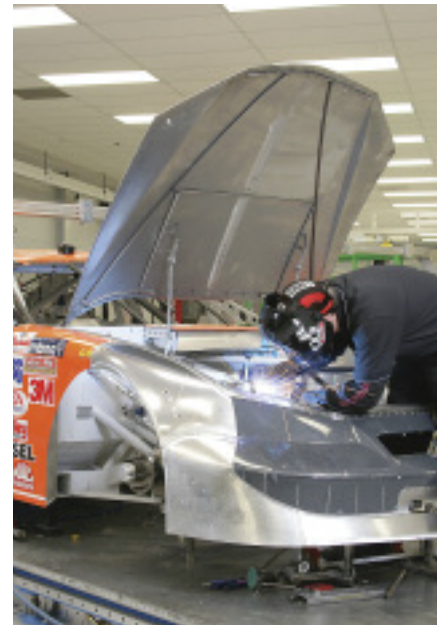
Chrome-moly is now being used in some chassis extension components at Joe Gibbs Racing.
