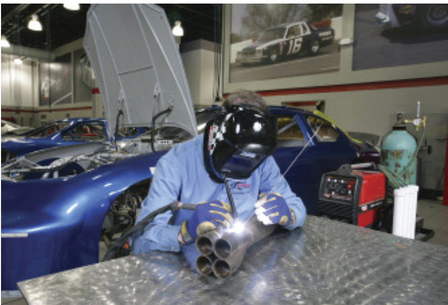
A welder uses an inverter-based gas tungsten arc welding machine on exhaust headers at Penske South Racing.
