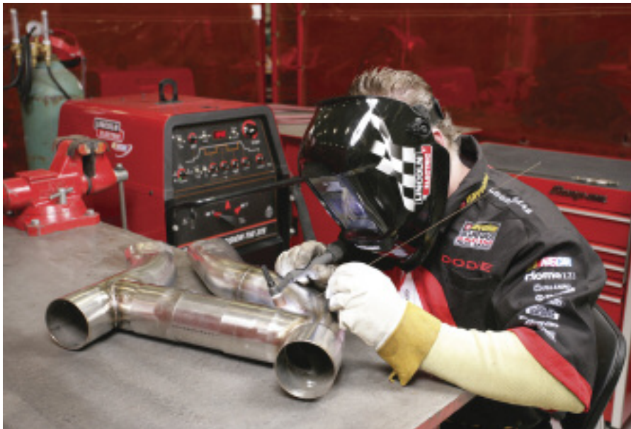
Fabricators at Chip Ganassi Racing use GTAW to repair and customize Nextel Cup exhaust components.
