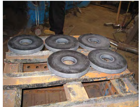
Individually as-forged weld wheels after forging operation was performed.
