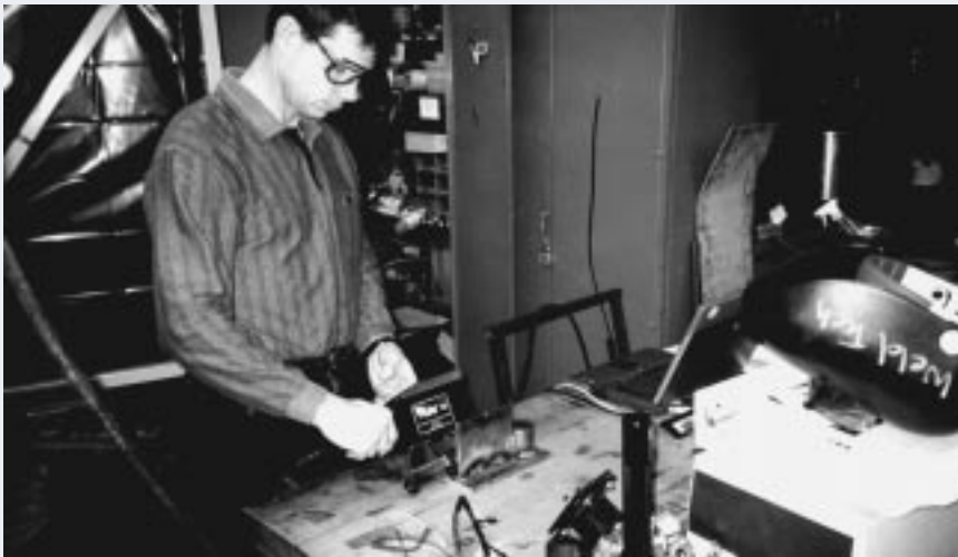
Fig. 2 — Jeff Noruk of Servo Robots using the LASER scanner to measure weld size and other discontinuities.
